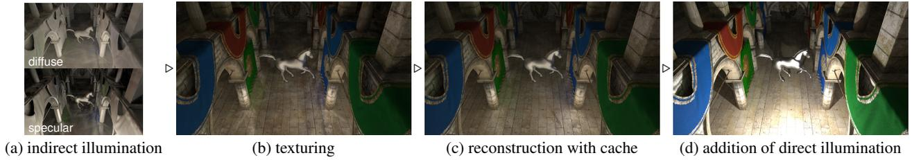
**Figure 3:** Processing flow of the final image computation (173961 triangles scene, 21 VPLs and 21 ray-bundles per frame). (a) Indirect illumination buffer is computed by bidirectional path tracing with spatial interleaved sampling and geometry-aware filter. (b) The indirect illumination is textured with diffuse maps and specular maps. (c) Reconstruction with the past indirect illumination performs anti-aliasing and error reduction. (d) The final image is obtained with direct illumination.
