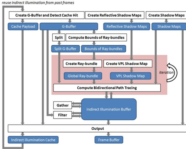
**Figure 2:** Rendering pipeline of our system. White blocks: procedures. Blue blocks: memory resources. Gray arrows: input-output relationship. Vertex buffer or texture maps are omitted from this figure to simplify. The procedures are executed in order from top to bottom in each frame.
