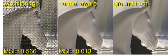
Figure D.2: Filtering diffuse indirect illumination. Our diffuse lobe-aware filtering is equivalent to the normal-aware filtering. The variance parameter is given as \sigma_n^2 = 0.05404477 when \beta = 20 and \kappa = 100 .
